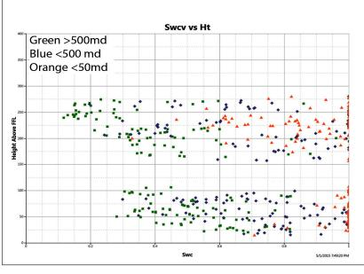
A plot of Sw vs K for two wells at different heights above the oil/ water contact is shown with permeability ranges color-coded (left). High-perm rocks have lower Sw than low-perm rocks. The spread of data to the right indicates depletion in some samples. This dataset demonstrates the influence of capillary pressure on reservoir saturations.
