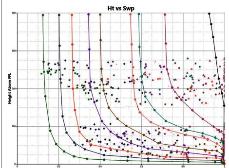
Then, fit a pseudo-capillary pressure curve to each group. Fit the curve to the low-Sw edge the dataset, and give it the characteristic shape of a capillary pressure curve. The plot (left) shows the full set of fitted curves color-coded to their permeability group. The log plot below illustrates the results of using the pseudo-Pc curves in a saturation model in the same way laboratory curves would be used.
