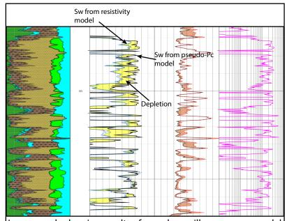
Log example showing results of pseudo-capillary pressure model compared to resistivity-based Sw
